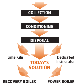
Cluster rule legislation requires kraft pulp mills to collect and incinerate HVLC NCGs.
