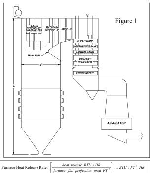
Let's review some of the fundamentals of typical USA boiler furnaces. Interestingly, the furnace volumes, heat release rates and literal tons of steel for a given capacity boiler are very similar. Most pre-CAAA pulverized coal designs are sized for a furnace heat release rate of between 75,000 - 85,000 Btu/ft²/hr.
